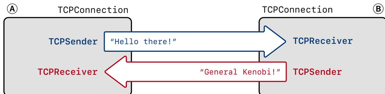
The two parties (“A” and “B” in the above diagram) are called the “endpoints” of the connection, or the “peers.” Your `TCPConnection` acts as *one* of the peers. It’s responsible for receiving and sending segments, making sure the sender and receiver are informed about and have a chance to contribute to *the fields they care about* for incoming and outgoing segments.
